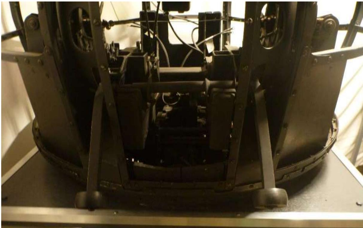
I managed to obtain sketches and patterns from the ever helpful Colin Waterworth and then started creating the missing parts. Firstly, two brackets were produced to do the job of the missing castings on the gun cradles. These were secured using the gun mount bolts to avoid drilling any further holes in the cradles.
