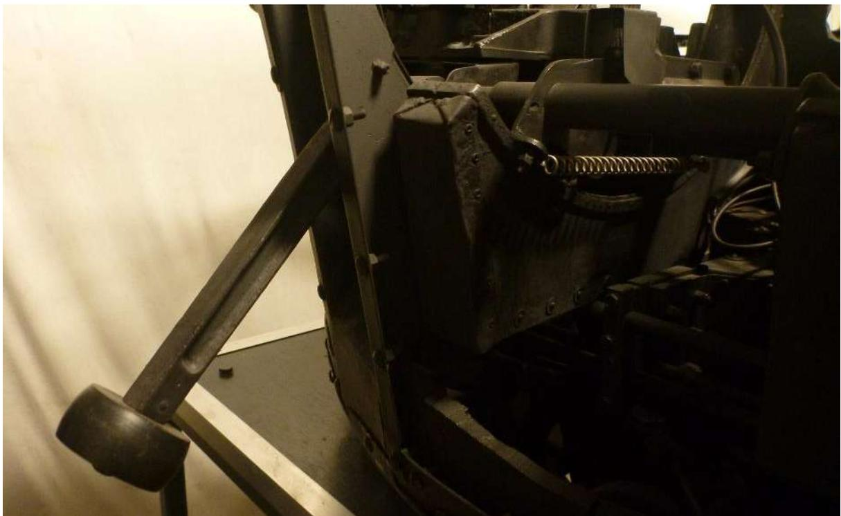
Then came the bracket to support the Bowden cable outers – made first in cardboard and then steel and fitted to the right hand gun cradle. The Bowden cables themselves are from a local bike shop. The staff asked what the cables I described were actually for and seemed mildly surprised when I replied “for a Lancaster mid-upper”. Luckily Bowden cables haven’t changed and a mountain bike brake cable does the job with a little bit of creative thinking.
