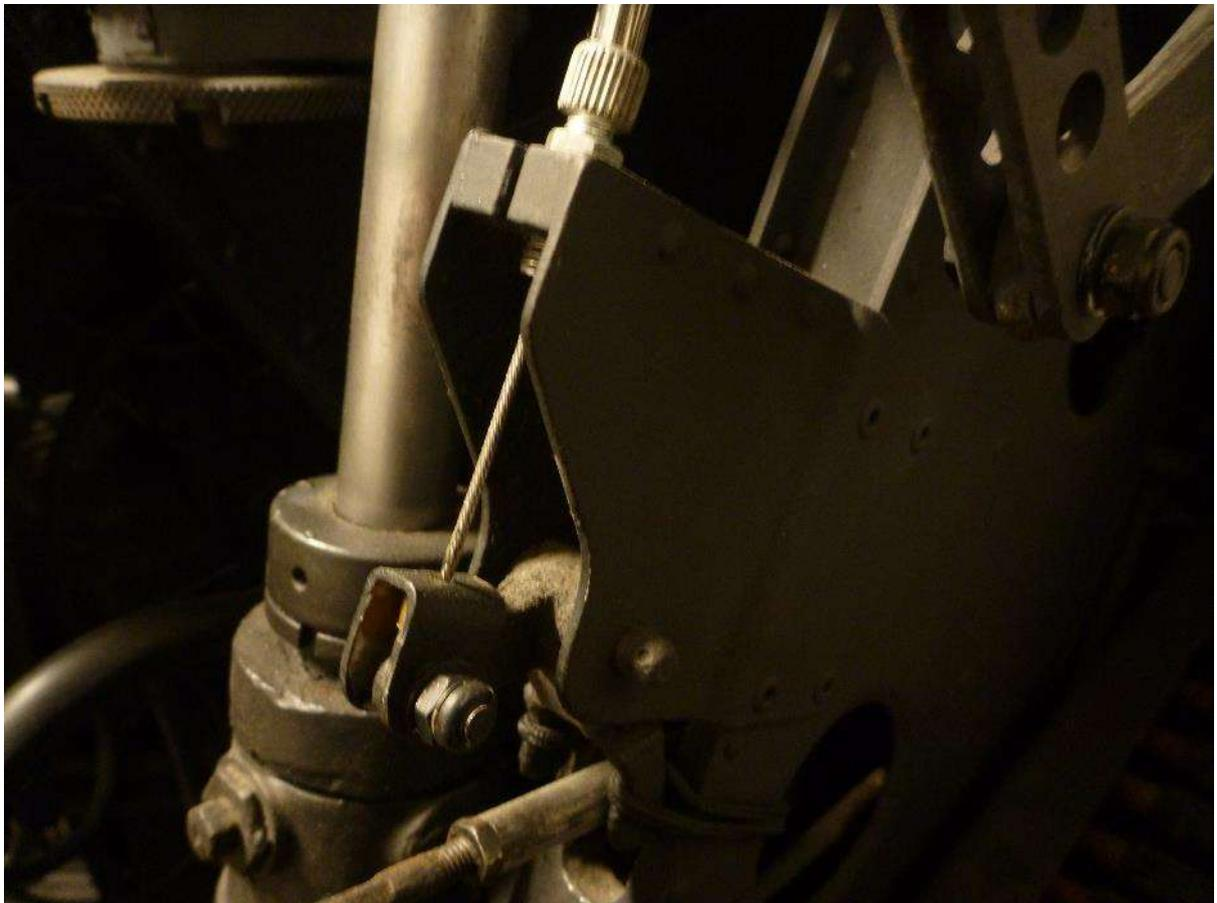
There was little to go on for the seat assembly either, but in this case I went to the schematic drawing in the various Air Publications. The right side detachable mount was fabricated from steel, whilst the seat "sling" was sewn up from an old RAF sausage bag. With the whole seat bolted in it was tried for size, adjusted a bit and then finally fitted.
